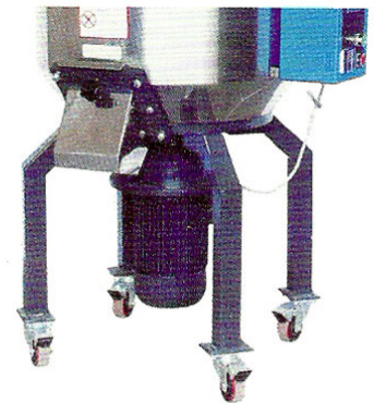
立式混色机可选配移动脚轮 IT CAN USE TRUNDLE FOR VERTICAL COLOR-MIXER
