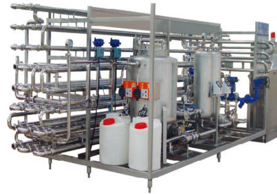
Pipe UHT sterilizer This sterilizer is mainly used for sterilization in high viscosity products with fiber and bigger flesh, and other products with high acidity, such as fruit juice, jam, coffee beverage, sterilized milk. Sterilization temperature is at 80°C-140°C. Capacity: 3T/H-15T/H.
